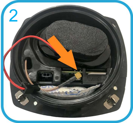
Carefully disconnect the internal antenna
