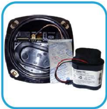
Remove old battery and desiccant pack
