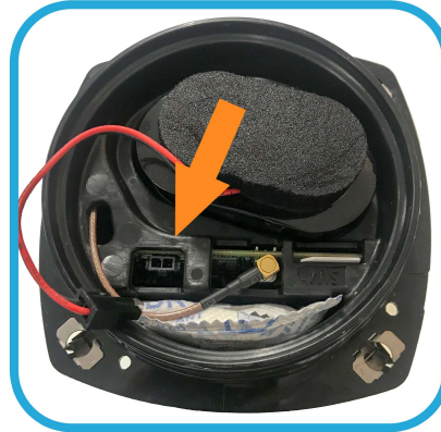
Carefully disconnect the battery cable
